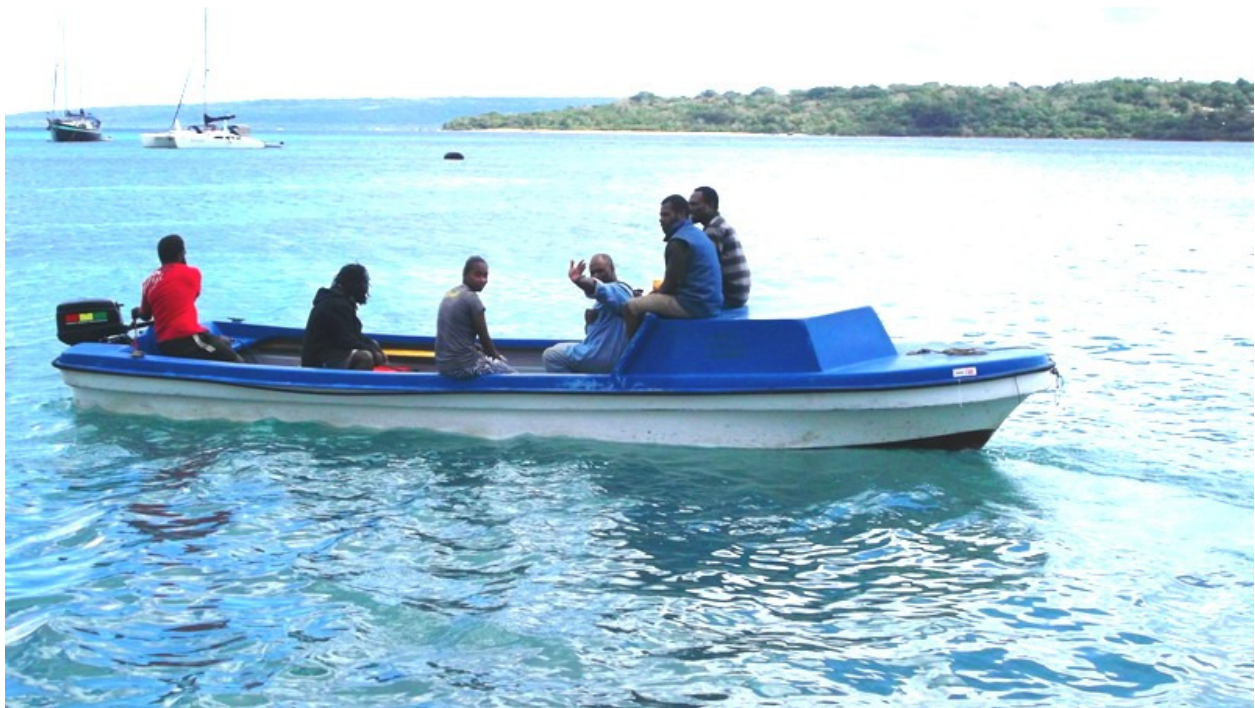
7m water taxi powered by HMI 15 HP engine with low pitch propeller
