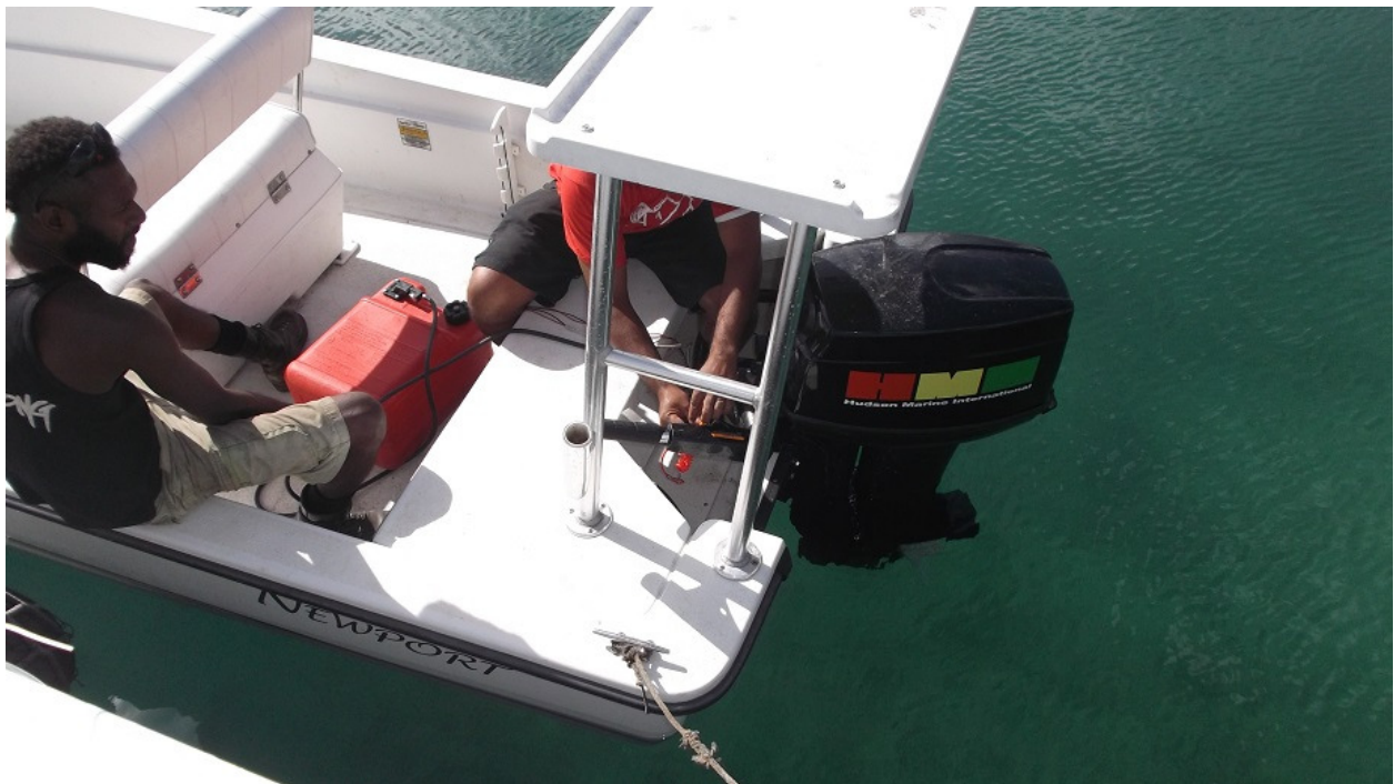
HMI OBM being connected to fuel tank
